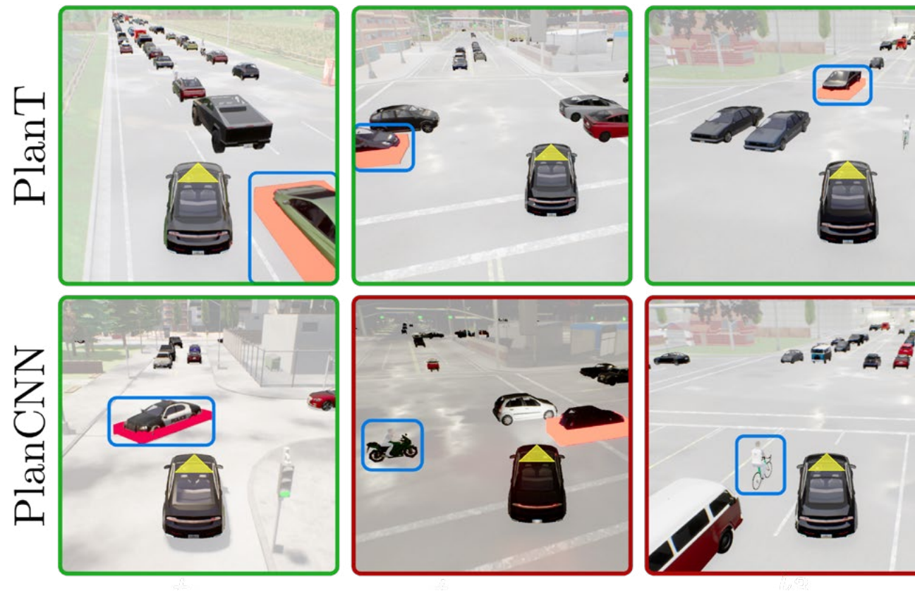
PlanT can drive safely in urban environments and in addition we can visualize on which vehicles the decision was based on. Vehicles with the highest relevance score are marked with a red bounding rectangle. We show examples for successful matching of relevance score and intuition (green frames) and failures (red frames). (© University of Tübingen)
