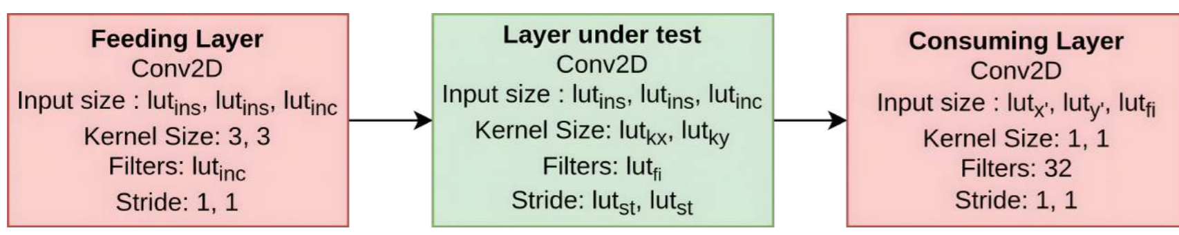
Figure 3: Preparation of the characterization process. A layer must be characterized without a „real“ network surrounding it. This leads to inaccuracies in the measured execution time due to optimizations and caching in the network compilation
